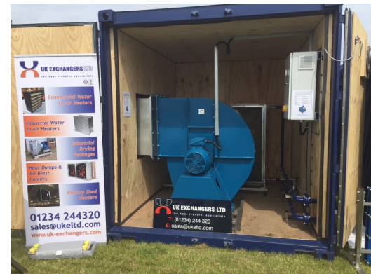
250 kW - G model in fully insulated container
