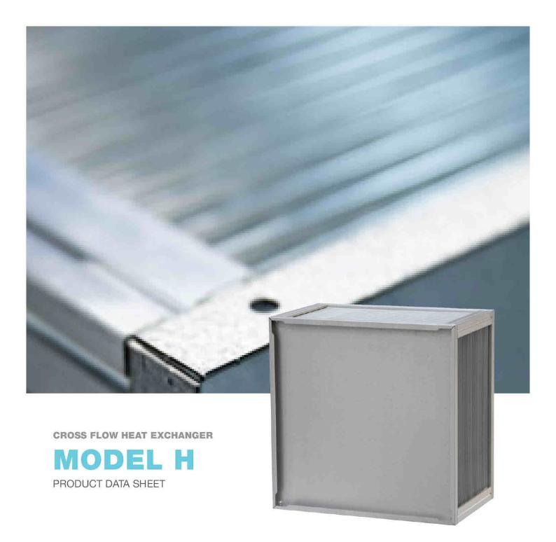
Model H is a high-performance, low-weight, crossflow plate heat exchanger with typical dry temperature efficiency up to 65% for single pass and 85% for two-step arrangements. The efficiency is improved by a unique plate design creating turbulence even at lower velocities. The strong aluminium plates in high standard alloy gives the products a long life time and with no moving parts the maintenance and service costs can be kept to a minimum.
